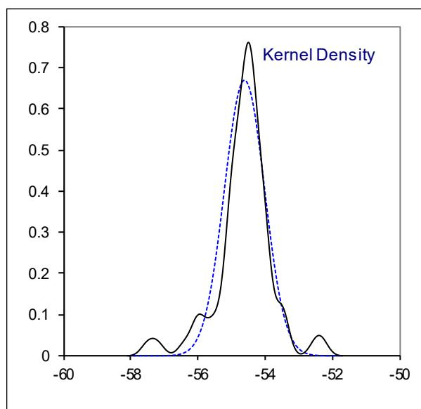
Determination of Kinematic Viscosity at -20°C on sample #20020; results in mm<sup>2</sup>/s
