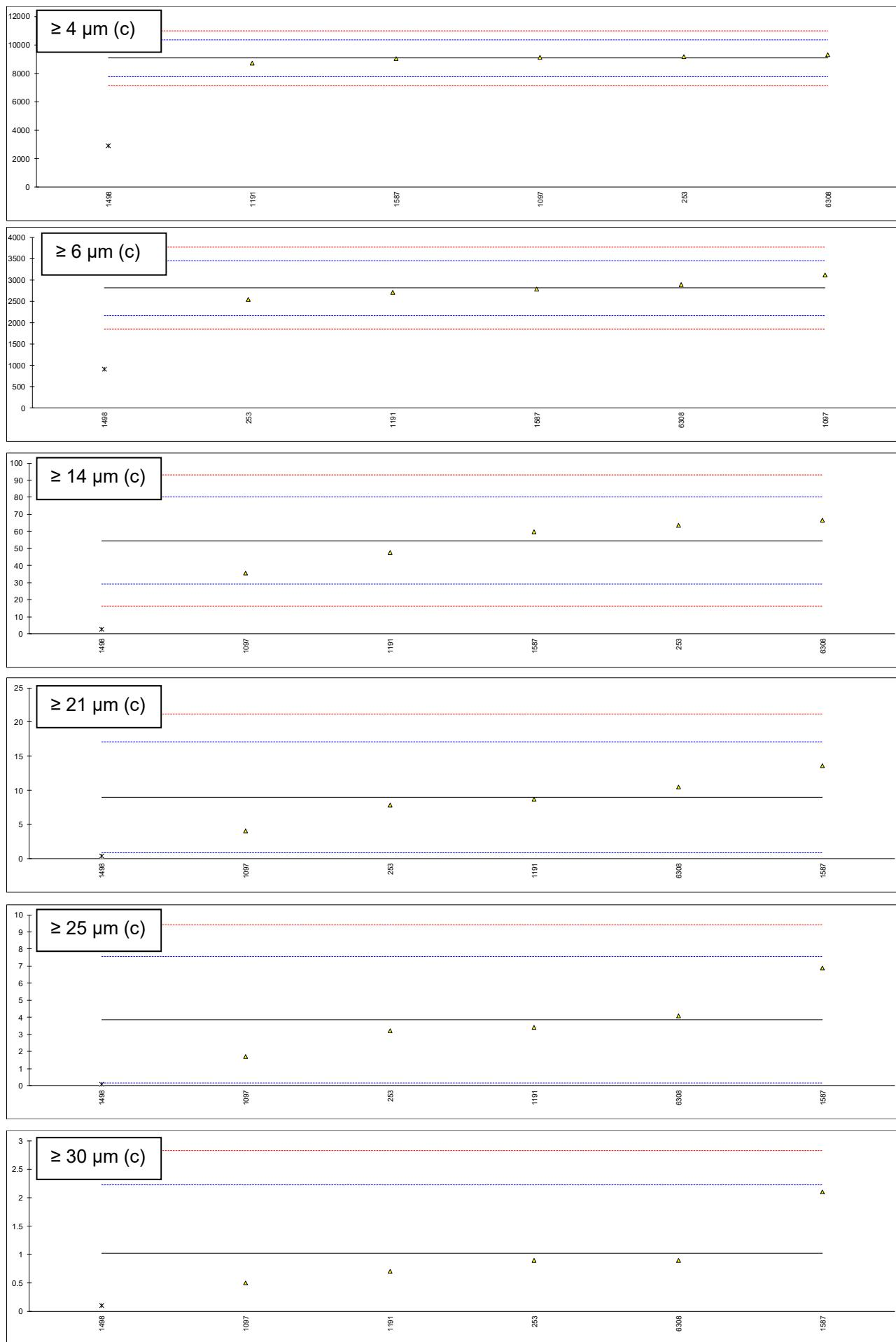
Determination of Particle Size Distribution by IP564 on sample #20021, results in ISO scale numbers
