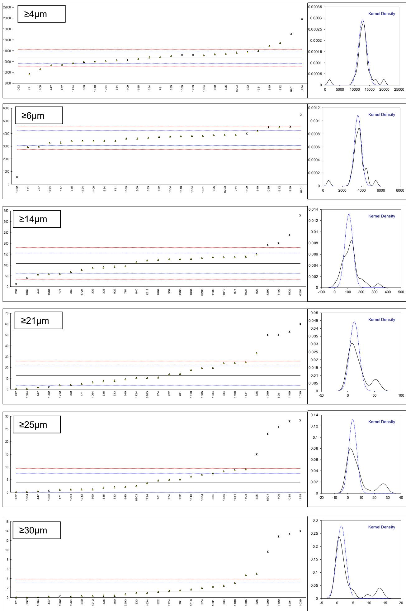
Determination of Particle Size Distribution by IP565 on sample #20021, results in ISO scale numbers
